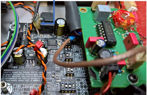
Both cables soldered direct to the PCB
